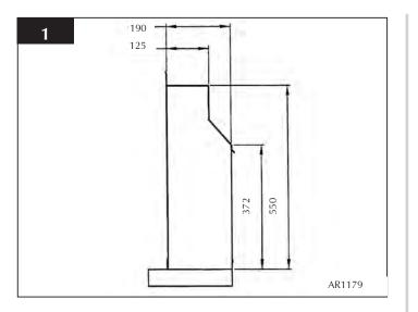
MINIMUM DEBRIS COLLECTION SPACE REQUIREMENTS-(EXISTING MASONRY CHIMNEYS ONLY) OVERALL EXTERNAL DIMENSIONS SIDE VIEW
